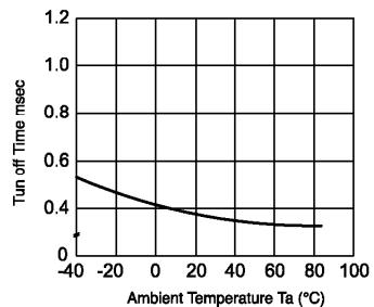
**Fig.5** LED operate vs. ambient temperature
